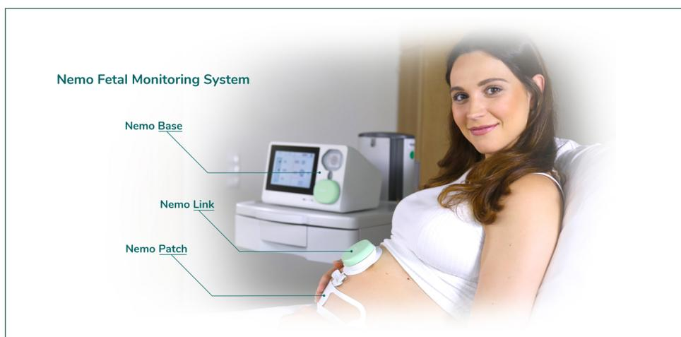
The NFMS uses a dedicated, multi-surface electrode patch with 6 electrodes. Fetal and maternal heart rate are derived from the recorded combined ECG-signals, and uterine activity is derived from the EMG-signals when the uterine muscles contract. Proprietary algorithms in the Nemo Base convert the amplified and wirelessly transmitted electrophysiological signals from the Nemo Link to readable information as is normally visualised on the central monitoring system of the hospital.
